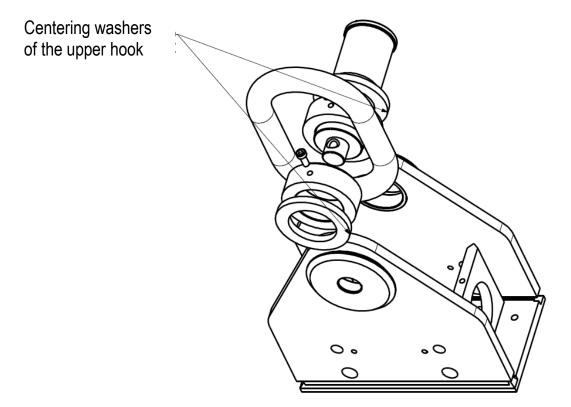
Insert the swiveling hook in the lower pivot with its centering washers as shown in the next figure:
