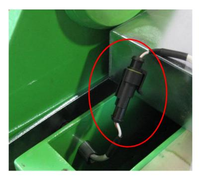
4) Unplug the AMP automotive connector from the battery pack.
