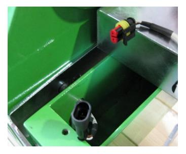
5) Connect the charger to the battery pack through the AMP automotive connector.
